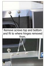
Remove the Hinge Plate from the top of the oven and fit diagonally opposite, to the lower corner.
